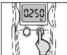
Press the **Memory** button to view the last 5 measurements. These are displayed for 20 seconds, after which the unit switches off.
