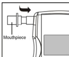
Insert a mouthpiece into the mouthpiece nozzle of the device.
